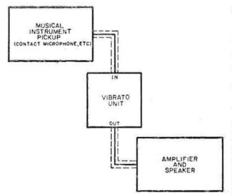
Block diagram shows correct interconnection of the three basic components of the revised setup. Use shielded microphone cable between units to prevent electrostatic hum pickup. If there seems to be excessive 60-cycle hum present, try reversing line plug of either amplifier or vibrato unit.
