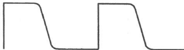
Fig. 2a. Waveform of the output signal
